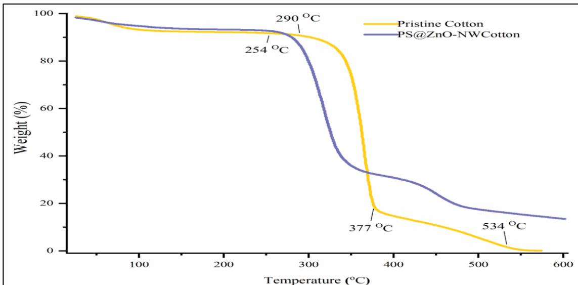
Fig. 8: Thermogravimetric analysis of pristine NWCotton and PS@ZnO-NWCotton.
