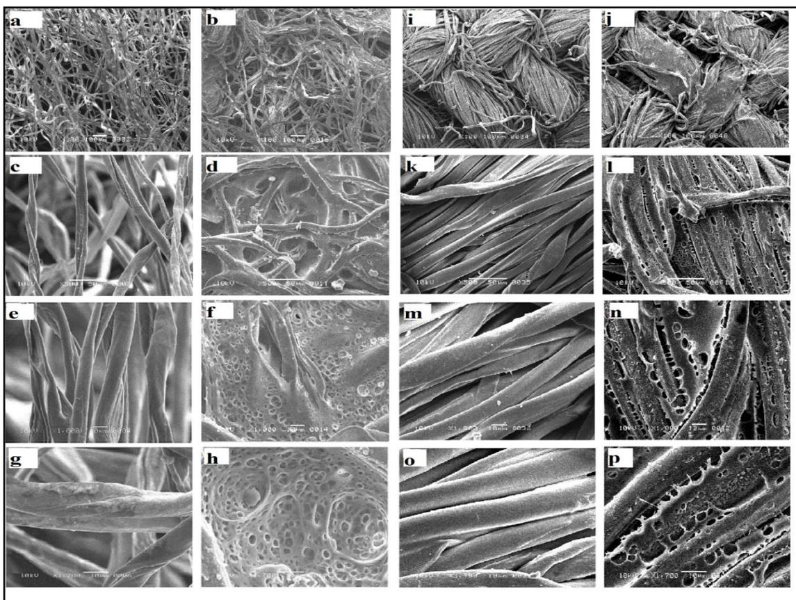
Fig. 7: Scanning Electron Microscopic images of pristine NWCotton (a, c, e, g), PS@ZnO-NWCotton composite (b, d, f, h)), Pristine WCotton (i,k,m,o) and PS@ZnO-WCotton (i,l,n,p) at x100, x500, x1000 and x1700 magnification.
