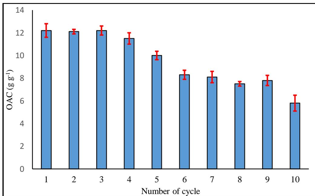
Fig. 11: Reusability of PS@ZnO-NWCotton for the adsorption of coconut oil up to ten cycles.
