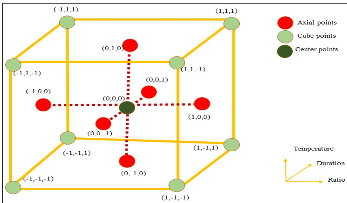
Fig. 1: Central Composite Design (CCD) of PS@ZnO-NWCotton composite, the dark green circles represent the center point, light green circles represent the cube points and red color represents axial points.
