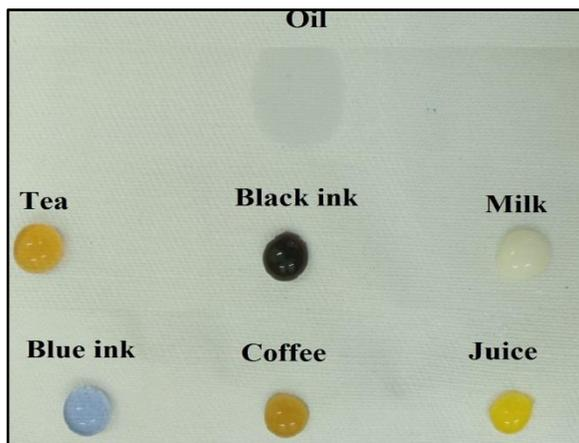
Fig 3: Common household liquids droplets on PS@ZnO-WCotton demonstrating its hydrophobic/ oleophilic properties.
