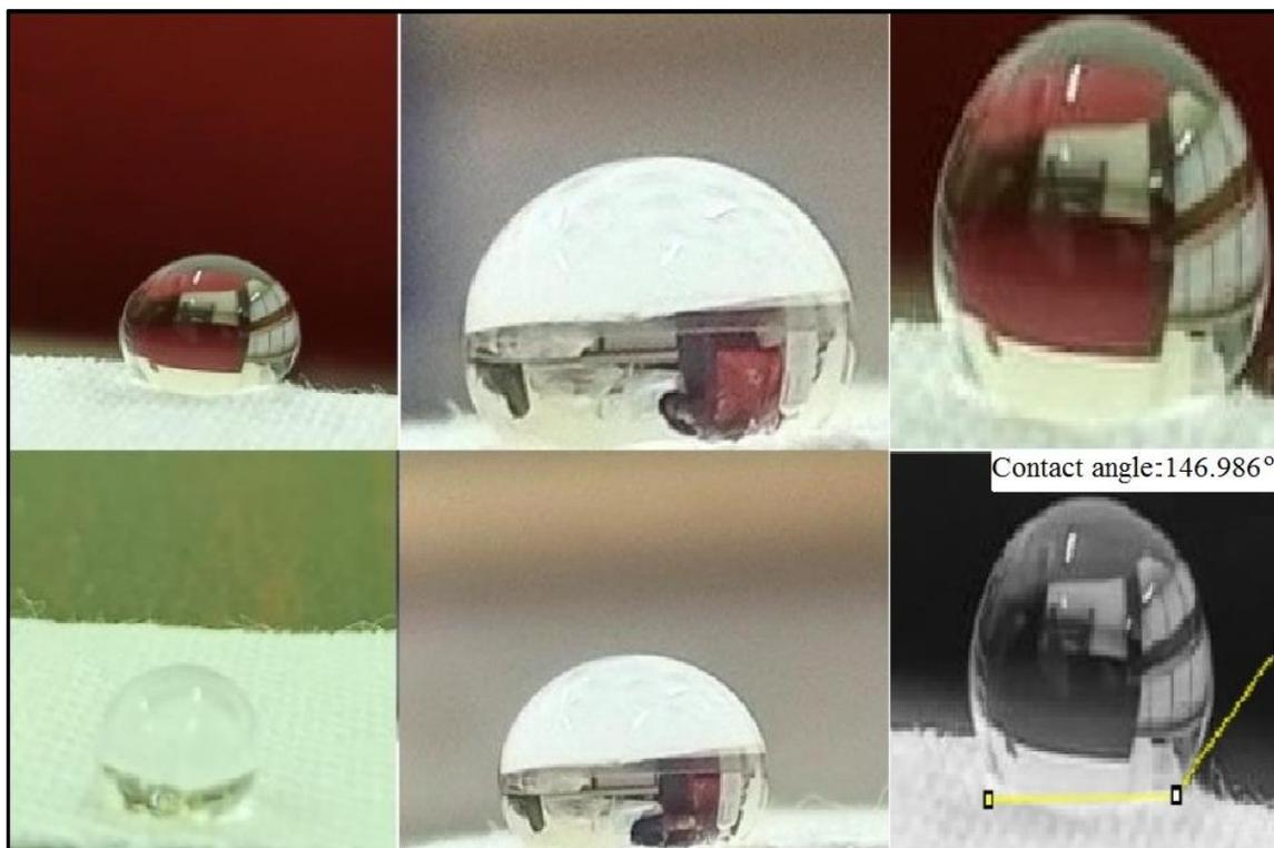
Fig. 5: Droplets of water on PS@ZnO-WCotton Composite used to determine contact angle.
