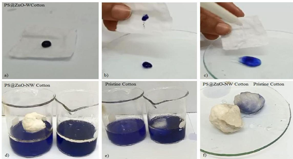
Fig. 4: (a) Spherical droplet of blue dyed water onto PS@ZnO-WCotton; (b) water droplet rolled off from PS@ZnO-WCotton surface by tilting it (c) adhered water was easily rinsed off without leaving any stain (d-e) illustrates adsorption of oil from dyed oil water mixture (water was dyed with blue ink). (d) PS@ZnO-NWCotton (e) pristine cotton (f) and PS@ZnO-NW Cotton and pristine cotton after 24 second immersion in dyed oil water mixture).
