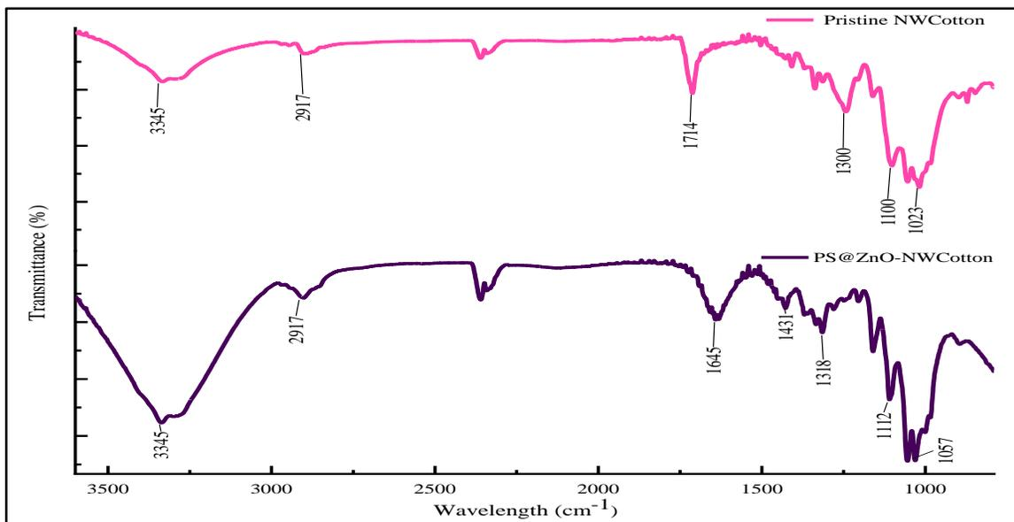
Fig. 6: FTIR spectra of Pristine NWCotton and PS@ZnO-NWCotton Composite.
