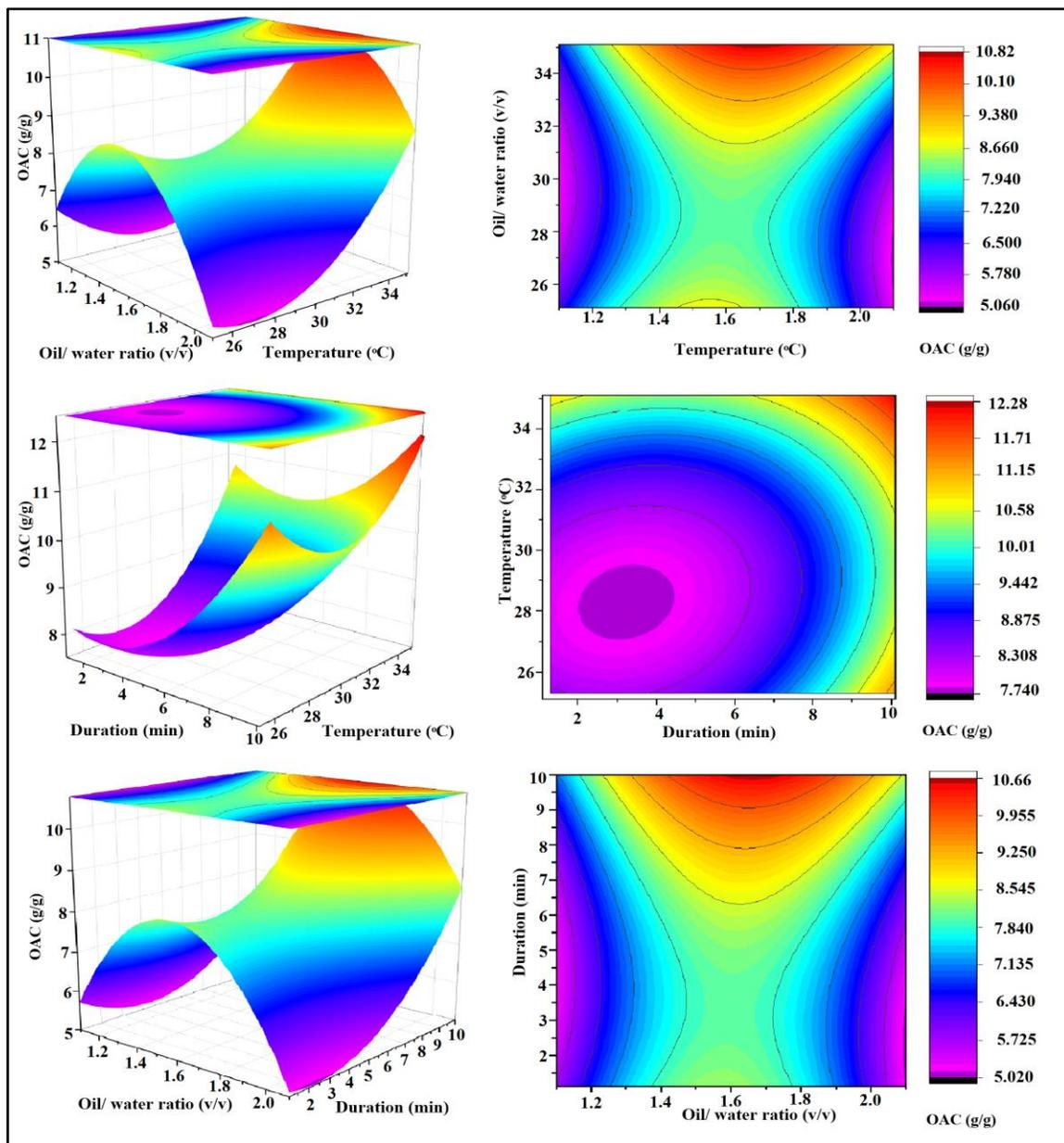
Fig. 10: 3D Surface response and contour plots for the adsorption of coconut oil onto PS@ZnO-NWCotton (a) OAC (g/g) versus temperature (°C) and oil/water ratio (b) OAC (g/g) versus duration (min) and temperature (°C) (c) OAC (g/g) versus oil/water ratio and duration (min).
